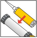
4. Place the cartridge into the gun and start applicatio
