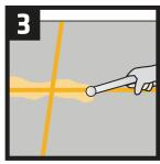
After 6 to 8 hours, remove any excess product on the tile with a sharp scraper
