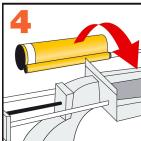
When the work is interrupted the static mixer nozzle can remain on the cartridge after the gun pressure has been released. If the resin has hardened in the nozzle
