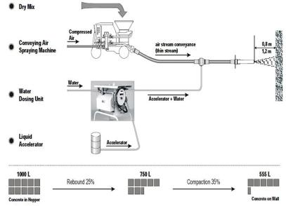
**Wet process:** Sika® Sigunit® L-1453 AF is supplied from the liquid dosing unit to the mixing tube assembly by means of air under pressure (2-3 bars more than the conveying pressure). The mixing tube assembly being located ~2.5 meters behind the nozzle or at the nozzle directly.
