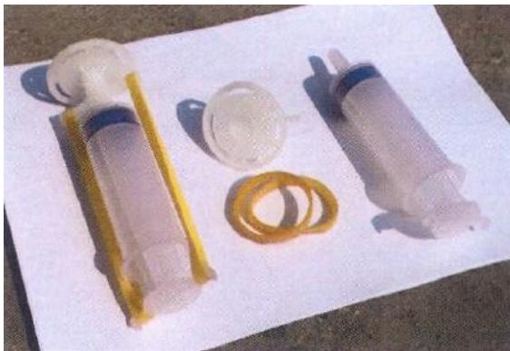
Injection tools: cylinders, plastic bowls, rubber bands
