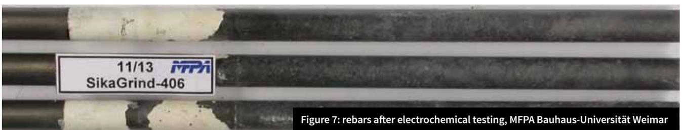
Figure 7: rebars after electrochemical testing, MFPA Bauhaus-Universität Weimar
