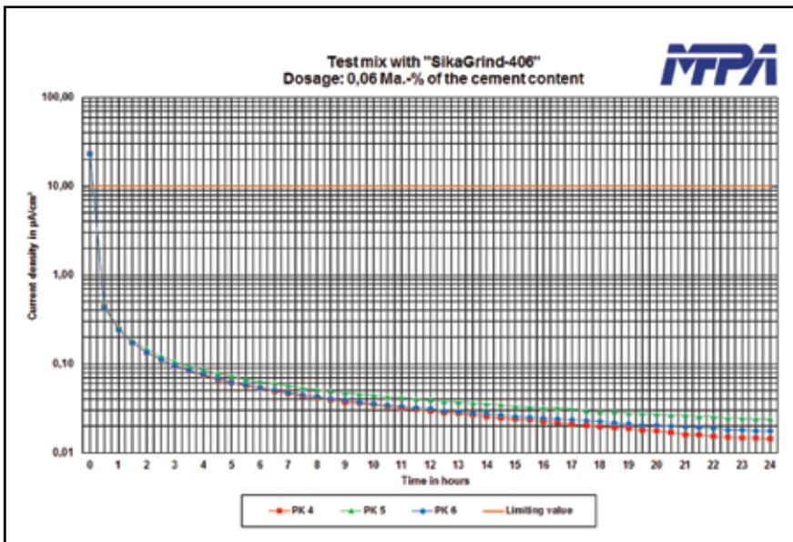
Figure 6: electrochemical test according to EN 480-14:2007-03, MFPA Bauhaus-Universität Weimar
